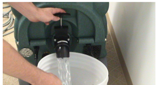
Draining the Recovery Tank
